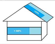
For any of the above situations, the wall thickness and insulation can match the existing wall cavity, to a minimum of 2x4" R14 nominal (RSI 2.5 W/m2K), and the existing roof cavity to a minimum of 2x6" R22 nominal (RSI 3.87 W/m2K) If insulation is being added, proper moisture and weather barriers must be installed per VBBL Section 9.25
