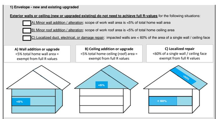
For any of the above situations, the wall thickness and insulation <u>can match the existing wall cavity</u>, to a minimum of 2x4" R14 nominal (RSI 2.5 W/m2K), and <u>the existing roof cavity</u> to a minimum of 2x6" R22 nominal (RSI 3.87 W/m2K) If insulation is being added, proper moisture and weather barriers must be installed per VBBL Section 9.25
